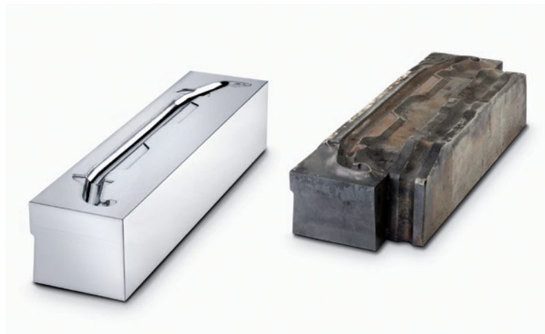
Cleaned and reconditioned forge tool
