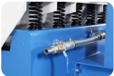
Dirty Water Discharge Valve
