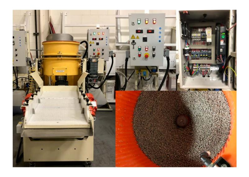
New machine. Disk finishing VKS 50L is a direct drive heavy duty machine. Equipped with VFD, programmable timer, dosing pump, solenoid valve/water feed. Unloading of machine/tilting is done via el.motor/gear box.
