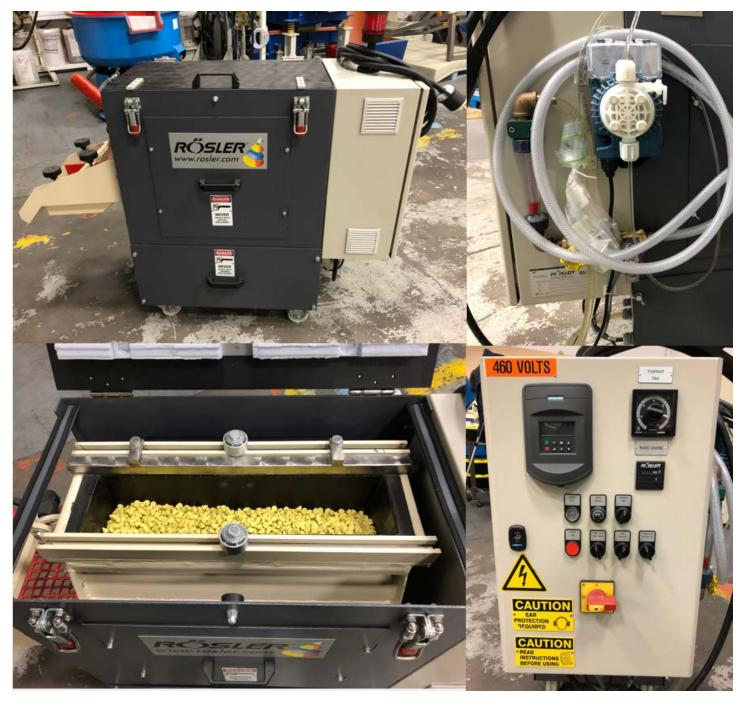
New machine. Rosler 18L (18cmx53cm channel) 3000rpm is full process machine. Equipped with VFD, sound cover, mobile frame, one divider, process timer, large water bar, dosing pump, water flow control, solenoid valve and many extras. It is a very versatile, 3000rpm tub, highly applicable for deburring, smoothing and polishing of the AM3D, medical and aerospace parts. Applicable for processing of the all metal, plastic, rubber parts... 400/460VAC 3 phase machine.
