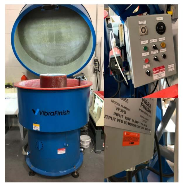
Type – Round vibratory bowl/flat bottom, 3 cubic feet, 10" channel width, bowl diameter 39" complete process machine
