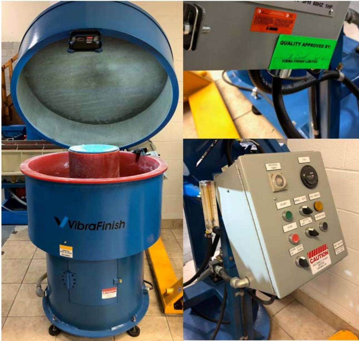
Type – Round vibratory bowl/flat bottom, 3 cubic feet, 10" channel width, bowl diameter 39" complete process machine
