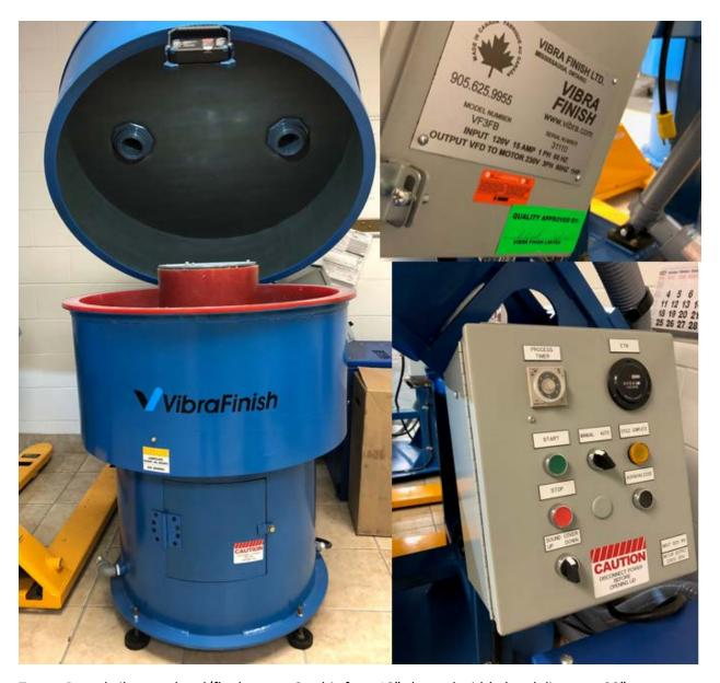
Type – Round vibratory bowl/flat bottom, 3 cubic feet, 10" channel width, bowl diameter 39"
