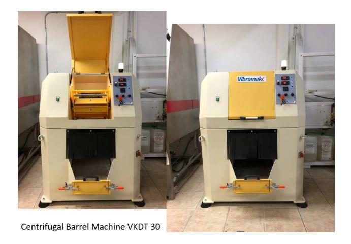
The VKDT 30 is a compact heavy duty deburring and polishing machine. Small medical, aerospace, or automotive parts can be finished using multiple steps. These machines are also excellent in the 3D printing industry for improving surface Ra - to below Ra 30 (in multiple steps).
