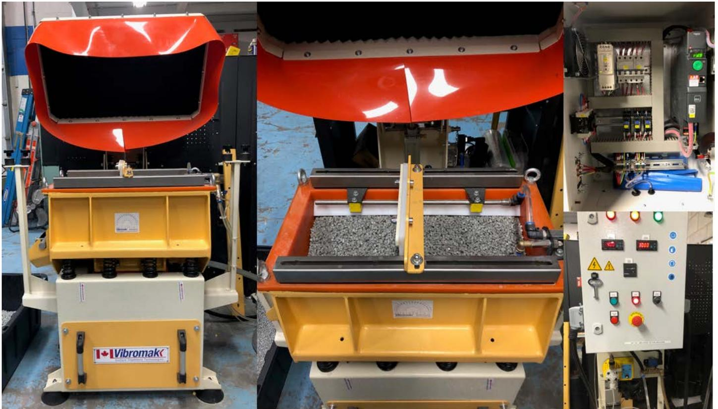
New machine. VKT 30 Liters/1Cu.ft 3000 rpm vibratory finishing tub is equipped with pneumatic sound cover, one divider, triangular wedge (for easy turning of the light parts), compound dosing pump, VFD, one SST drain, solenoid valve for water feed, cross bar for individual clamping/fixing of the parts etc.... It is built for processing (deburring, smoothing and polishing) of the AM3D parts, aerospace blades and airfoils, medical machined and 3D parts etc... Highly versatile machine.
